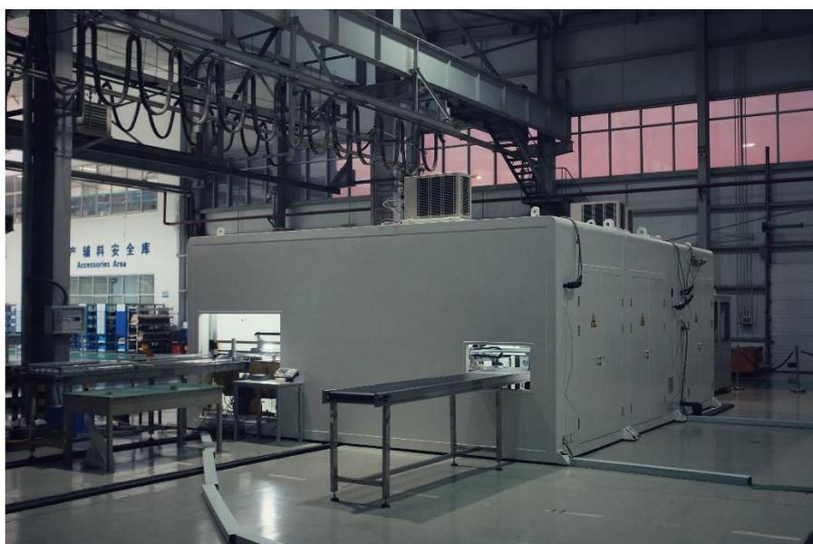
PhotonAssay unit as seen from the front. The sample input and output are located on the left- and right-hand sides respectively
