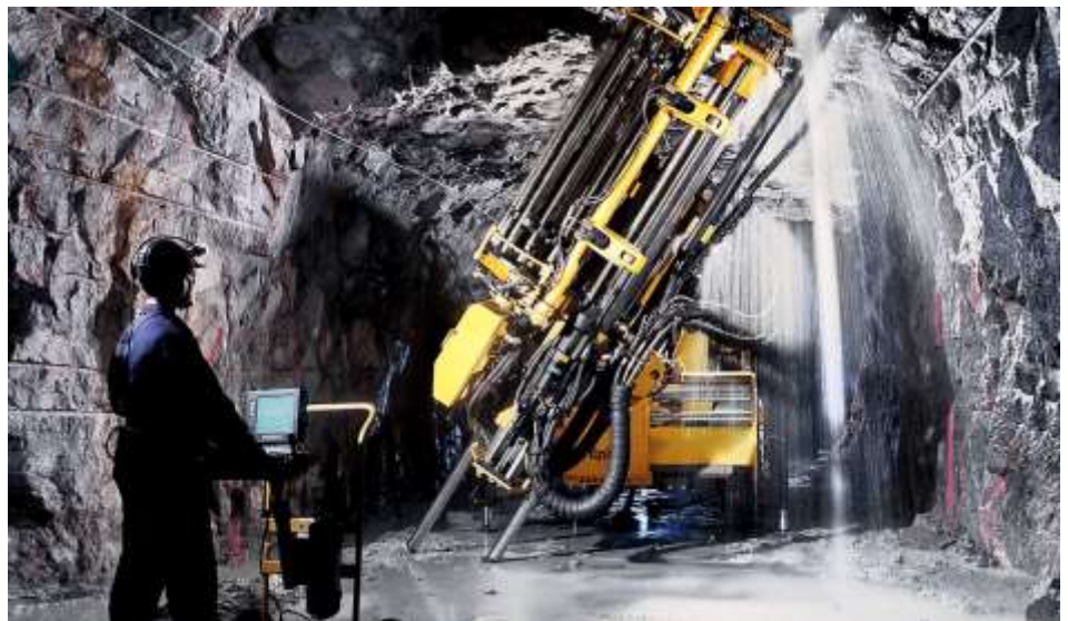
Figure 15: Simba M4 Underground Production Drill Rig
