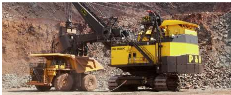
Figure 12: P&H 4100 Electric Rope Shovel
