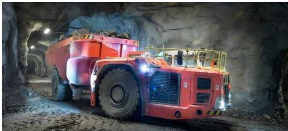
Figure 16: Sandvik TH663i Underground Haul Truck
