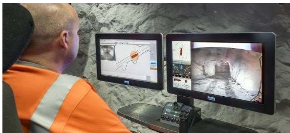
Figure 13: Sandvik AutoMine semi-autonomous control
