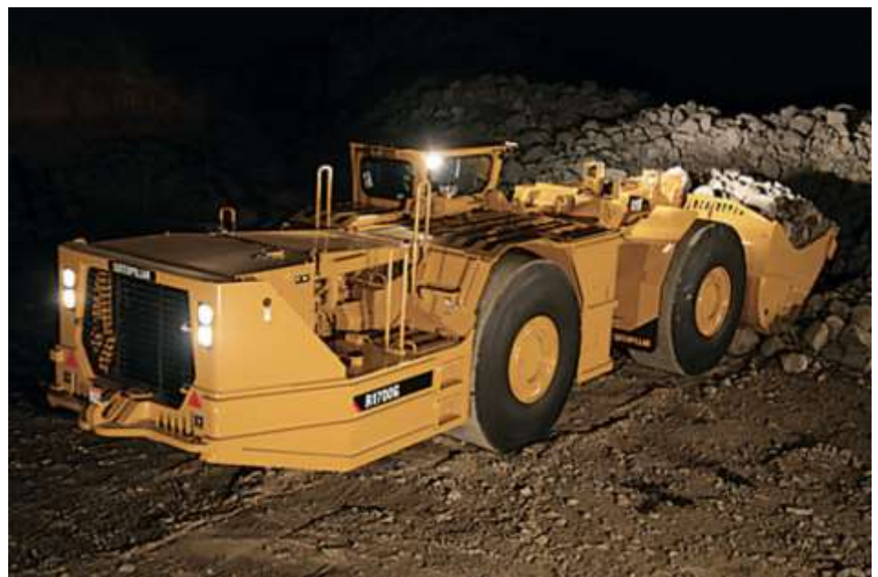
Figure 14: Caterpillar R1700G Underground LHD
