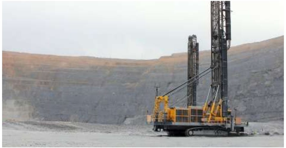
Figure 10: Epiroc Rotary Blast Drill Rig PV-351
