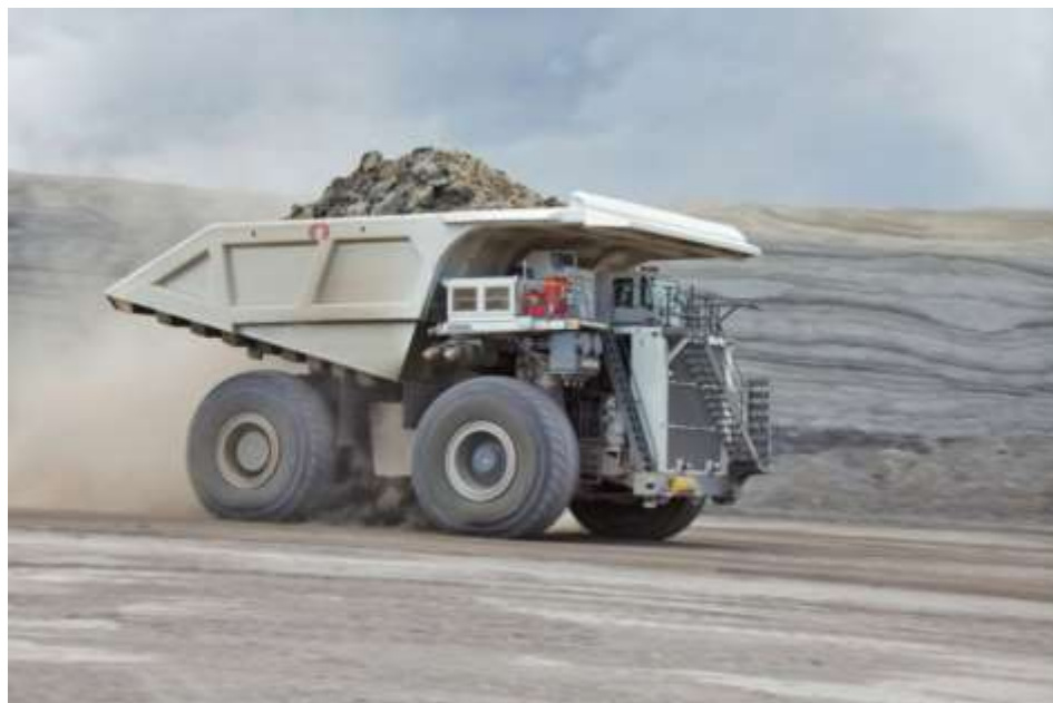
Figure 5: Liebherr T284 mining truck
