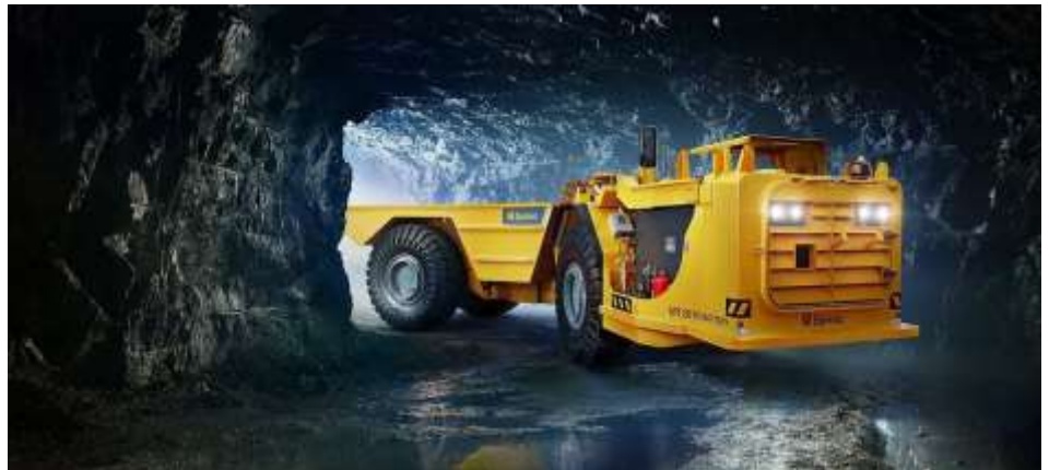
Figure 17: Epiroc Minetruck MT42 Battery
