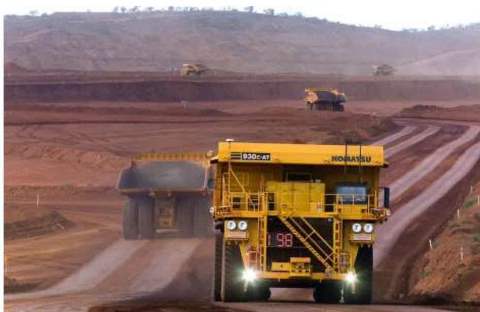
Figure 2: Komatsu 930E haul truck
