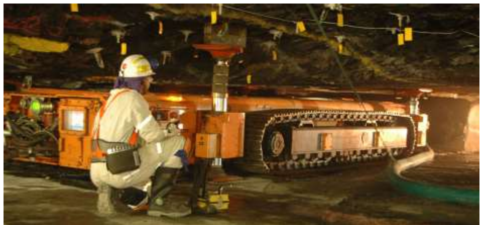
Figure 6: Anglo American's Rapid Mine Development System
